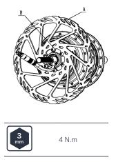
2. Install the freewheel (A) onto the motor axle from the right side, and tighten it.
