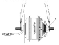
4. Install a 2 mm washer (A) onto the motor axle from the right side. Install a M12 cap nut (B), and tighten it.
