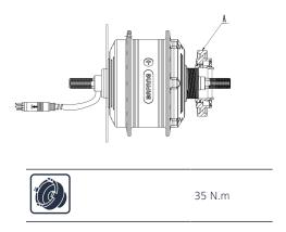
3. Install a non-turn washer (A) onto the motor axle from the right side, and insert the motor into the frame.
